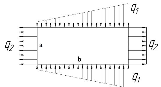
$$q_1 = 20 \text{ кН/м}, q_2 = 15 \text{ кН/м}, a = 3 \text{ м}, b = 8 \text{ м}$$
