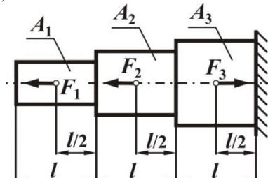
$F_1 = 20 \text{ kH}, F_2 = 25 \text{ kH}, F_3 = 40 \text{ kH}, l = 1 \text{ м}, A_1 = 100 \text{ мм}^2, A_2 = 200 \text{ мм}^2, A_3 = 300 \text{ мм}^2, E = 2 \cdot 10^5 \text{ Мпа}$ |
